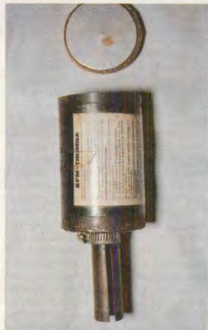
SFM grenade launcher: Cup-type designed to launch SFM 4 hand grenade, range 100 meters at 45 degrees, designed for use with 12-gauge shotguns, steel and felt disc protects grenade from muzzle blast.
